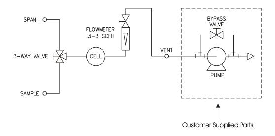
Figure 3-4: Piping Diagram for Vacuum Service Option
